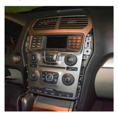
12. Refit all four retaining bolts removed in step 2 securing the console control panel as shown.
