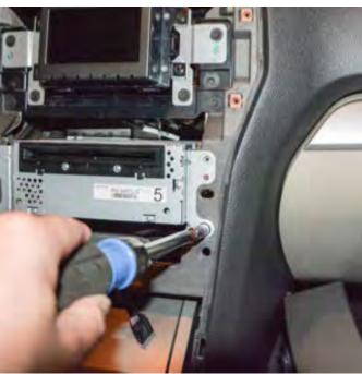
6. Align the right hand side plate as shown and refit the two bolts removed in step 5. Do not tighten
