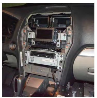
4. Disconnect the wiring harness.
