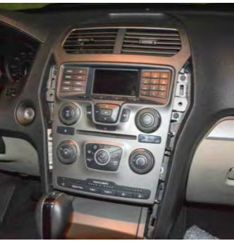
2. Remove all four retaining bolts securing the console control panel as shown.
